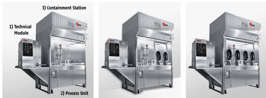
Glatt Containment Station (Barrier) can be executed in three configurations, shown above, (left to right): OCS Open Containment up to OEL 4; OCS with a sliding pane is fitted with glove ports to enable ergonomic working up to OEL 4/5; CCS Closed Containment System similar to Isolators and RABS, up to OEL 5.
