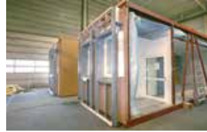
Each module has an individual steel frame
